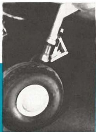
Hydraulic strut and 6.00 x 6 tire.
