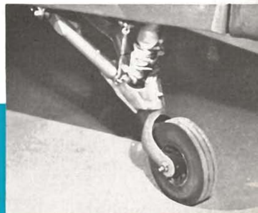
Shock-strut tail wheel.
